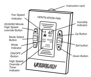
Connects to 3 wire 20 gauge low voltage wire
